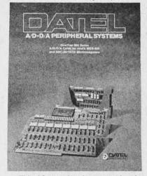
This 16 page brochure provides the specifications for the SineTrac 800 series of data acquisition cards for the Intel MDS-800 and SBC-80/20/10 microcomputers. Accepting 32 or more analog channels, the high speed SineTrac 800 communicates over the processor bus as an addressable IO device. The brochure is available from Datel Systems Inc, 1020 Turnpike St, Canton MA 02021, (617) 828-8000.
