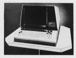
The Delta 4300E, a new video display terminal designed for text processing applications, features automatic word wrap, automatic ragged right sentence and paragraph justification, and automatic justification of new insertions.
